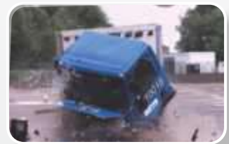
K4 Rated (6.8 Ton Truck Impacted at 48 km/h)
